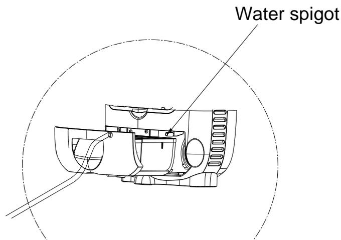
If you find that the water does not flow down the hose then check that it is running downhill, is not kinked, all excess tube has been cut off and is not blocked. If the water still does not flow then make a 4mm hole, 30mm from the spout in the top of the hose. This will balance out the air pressure and allow the water to flow.
